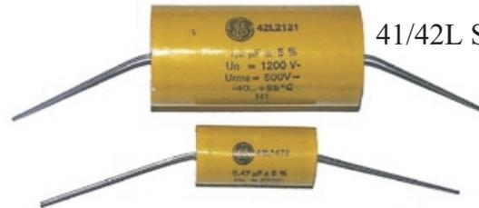
**GE 41L Series Metallized Polypropylene Capacitor;** axial; 5%; 40mm long tinned copper leads, yellow polyester wrapping with epoxy resin end fill; dissipation factor  $5 \times 10^{-4}$  @ 1KHz and 25°C; low ESR (series resistance)
