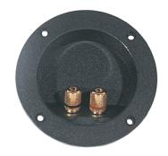
D-CUP Input Cup \$3.15 each All brass gold plated posts with knurled caps. Accepts banana plugs or 4 Awg wire. The cup is 4.14" round with a 3" round hole size.
