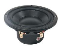
Znom ohm 6.2 Re ohm Le@1kHz 0.25 mH fs 72 Qms 3.13 Qes 1.03 Qts 0.75 5.54 q Mms Cms 0.84 mm/N
