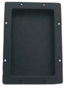
VL-CUP Input Cup \$1.40 each. Blank cup for mounting terminals and/or L-pads etc. 7" tall by 5" wide. Cut-out is 5.875" x 3.875". Available either blank or with 4 pair of 3/4" spaced holes drilled.
