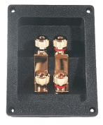
G25-CUP Input Cup \$5.50 each TD-CUP Input Cup \$8.10 each ribbed caps and straps for bi-wire applications. Accepts banana plugs or 4 Awg wire. The cup is 4.73" tall by 3.66" wide. Cut-out 3.7" x 2.9".
