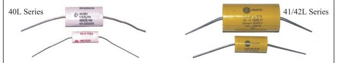
**GE 41L Series Metallized Polypropylene Capacitor**; axial; 5%; 40mm long tinned copper leads, yellow polyester wrapping with epoxy resin end fill; dissipation factor 5 x 10<sup>-4</sup> @ 1KHz and 25°C; low ESR (series resistance)
