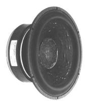
18W/8545K carbon/paper cone This 18W/8545K features a woofer. heavily damped and carbon fibre impregnated paper cone that dampens resonances normally associated with stiff cones. The magnet system is the new SD-1 system which eliminates modulation and dynamic distortion, as well as lowering clipping distortion created as the voice coil exceeds its maximum linear excursion. The "K"
