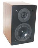
The Studio is a small monitor type speaker using the new Vifa XT ring radiator tweeter and the Vifa Premium Line 5" woofer. A 6" passive radiator is used on the back to tune the enclosure and extend the bass response. The frequency range is from 45Hz to 20kHz with very impressive bass for such a small speaker.
