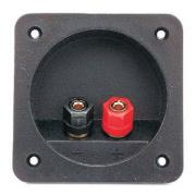
CB-CUP Input Cup \$1.55 each Chrome plated posts with plastic knobs and threaded inserts. Accepts banana plugs or 8 Awg. Wire. The cup is 3.15" square with a round 2.7" cut-out hole size.
