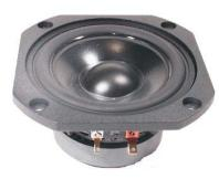
Znom ohm 6.29 ohm Re Le@1kHz .56 mH fs Hz Qms 3.20 Qes 0.54 Qts 0.45 Mms 5.49 g Cms mm/N
