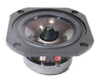
Znom ohm Re 6.4 ohm Le@1kHz 0.68 mH fs 70 Hz Qms 3.81 Qes 0.46 Qts 0.41 Mms 4.68 g Cms mm/N
