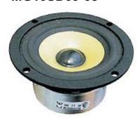
Znom ohm 5.5 ohm Re Le@1kHz 0.33 mH fs 81 Hz 3.40 Qms 0.73 Qes Qts 0.60 3.2 g Mms 0.48 Ns/m Rm
