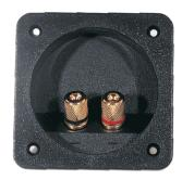
DB-CUP Input Cup \$3.15 each Gold plated posts with plastic knobs All brass gold plated posts with and threaded inserts. Accepts knurled caps. Accepts banana banana plugs or 8 Awg. wire. The plugs or 4 Awg wire. The cup is cup is 3.15" square with a round 3.15" square with a round 2.7" cut-out hole size.
